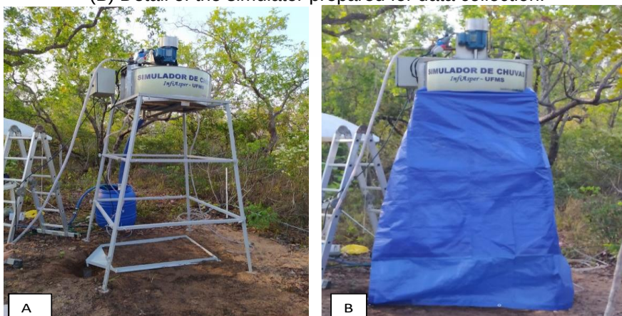
Figure 2. Rainfall simulator. (A) Detail of the simulator and the 0.70m 2 experimental plot and (B) Detail of the simulator prepared for data collection.
